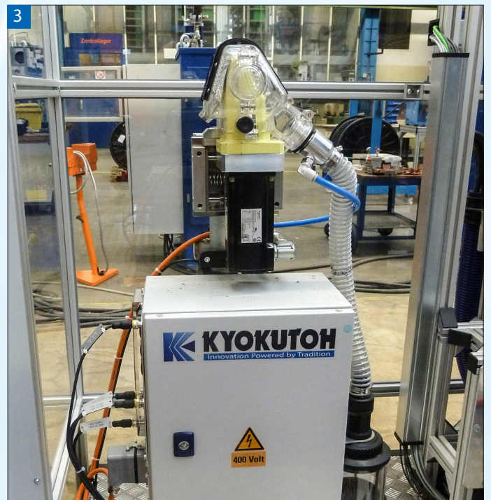
The KYOKUTOH tip dresser CD-EL with frequency converter, tuned to the welding process of the exhaust tract insulation.
